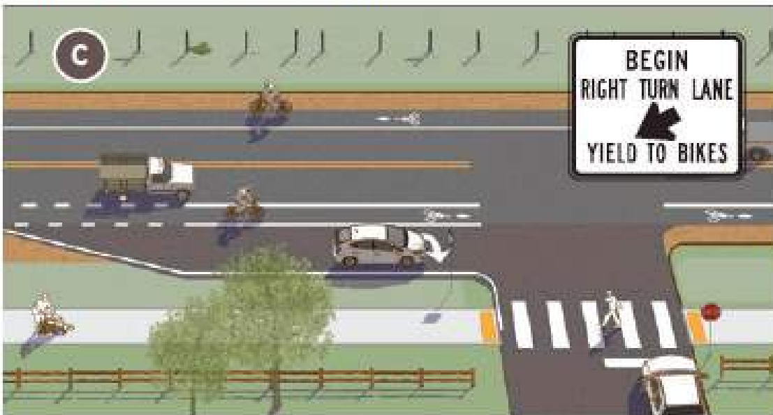
Figure 24: A variety of design treatments exist depending on the roadway configuration, available curb-to-curb width, traffic volumes and desire to provided a dedicated turn lane. All designs should strive to reduce speeds of turning vehicles, remind users of bicycle priority, and clarify user positioning approaching and through the intersection. Common signs at intersections include R4-4 "Begin Right Turn Lane Yield to Bikes" and a modified R10-15 "Turning Vehicles Yield to Bikes" sign.
